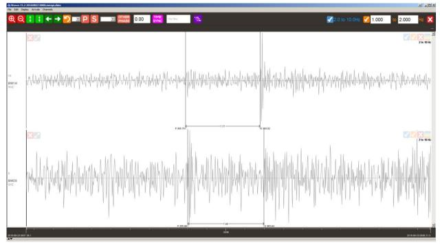
Figure 28: Record of an M1.3 Aftershock on BW1H and BW2S.
