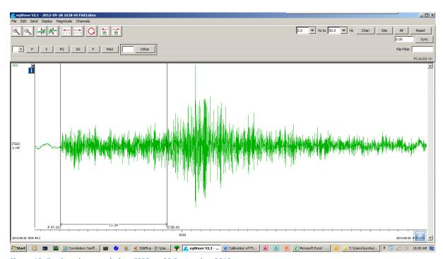
Figure 13: Earthquake recorded on FS03 on 28 September 2012.
